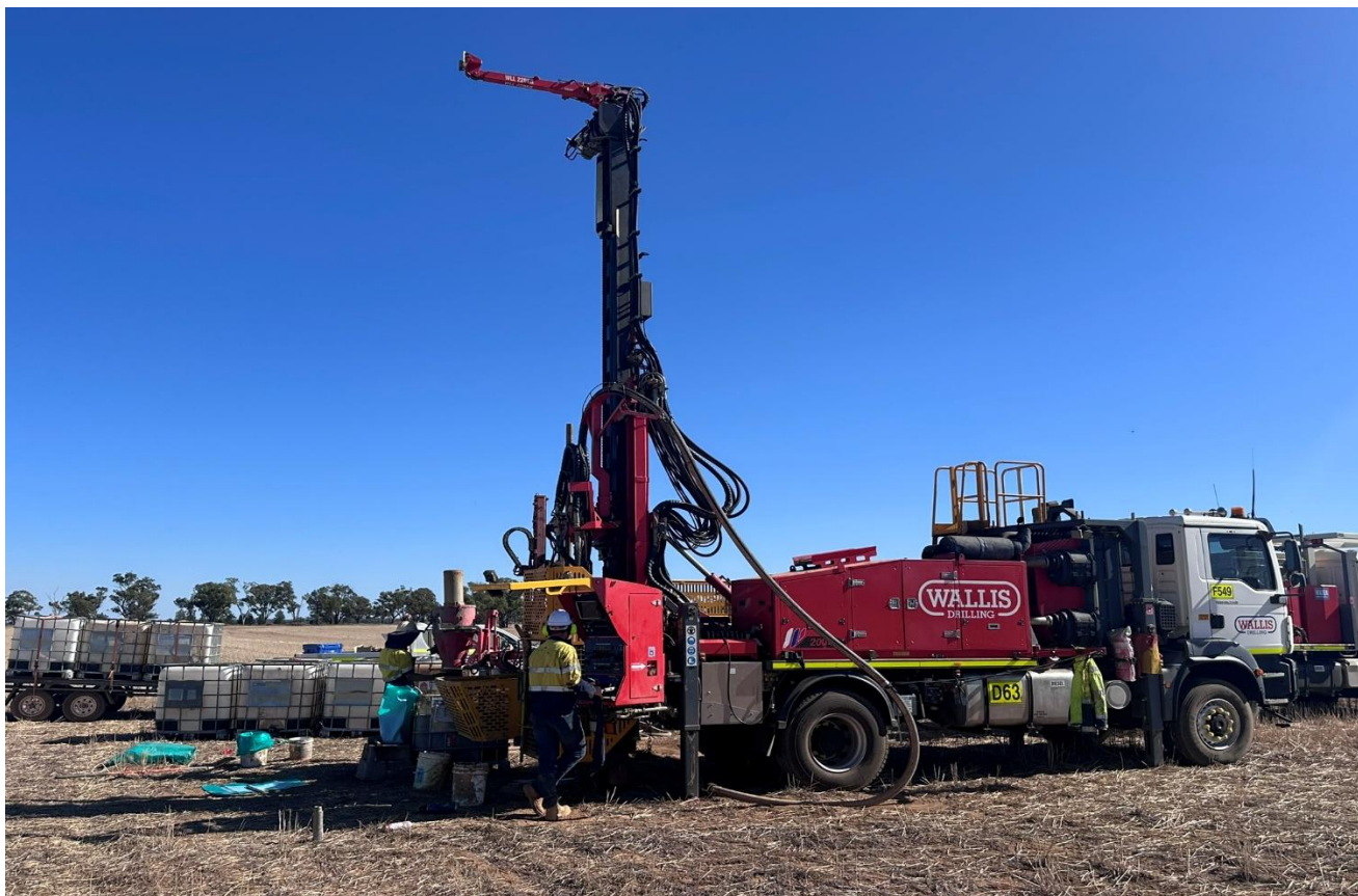
Figure 2: Trangie Air Core drilling being completed by contractor Wallis Drilling.
