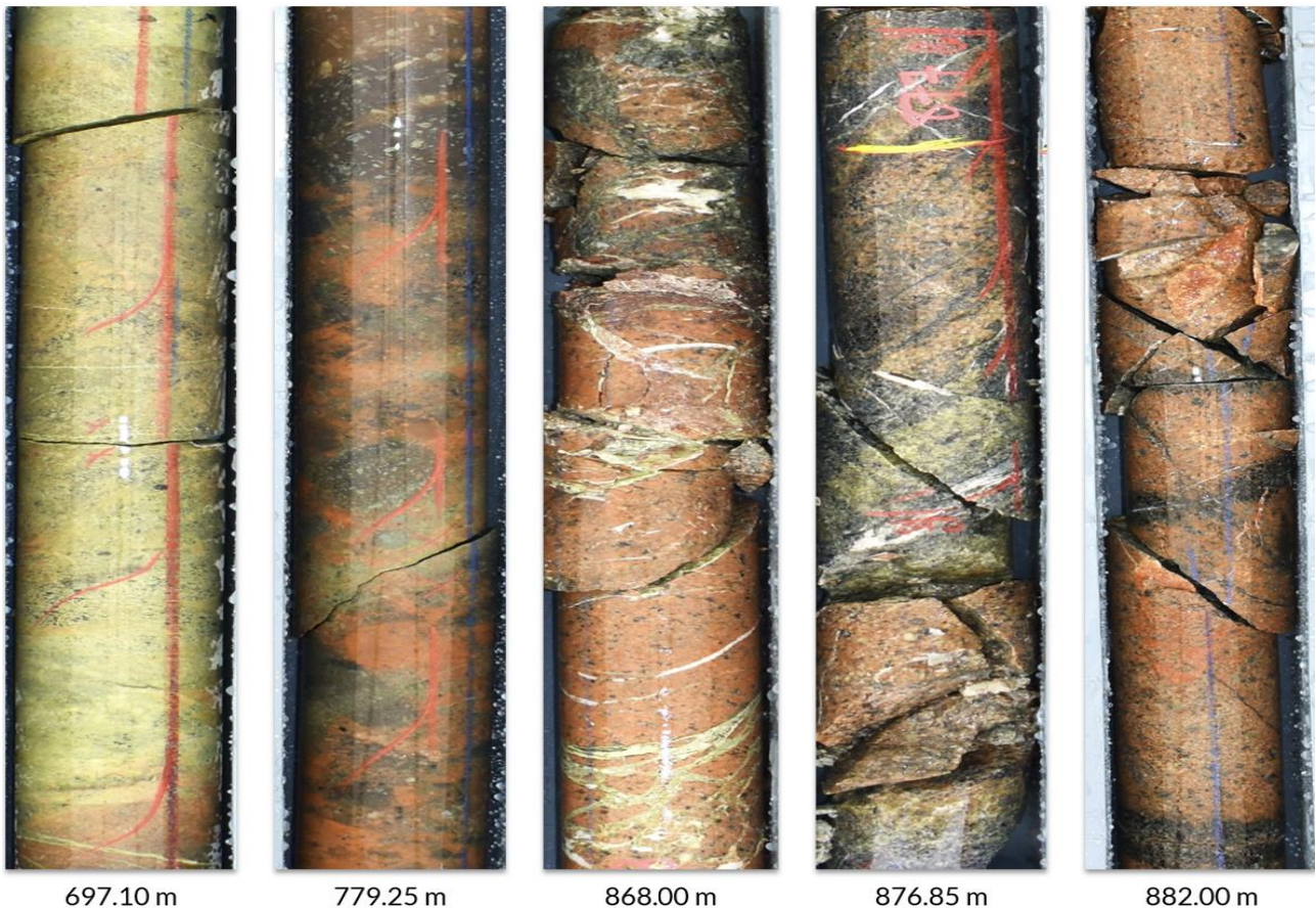
Figure 4: Select Duck Creek diamond drill core - Hole DCKDH017. Drilled to a depth of 895.1 metres in an east-north-easterly direction (080°) and a dip of -70°. NQ sized core shows a variety of different inner propylitic alteration styles.
