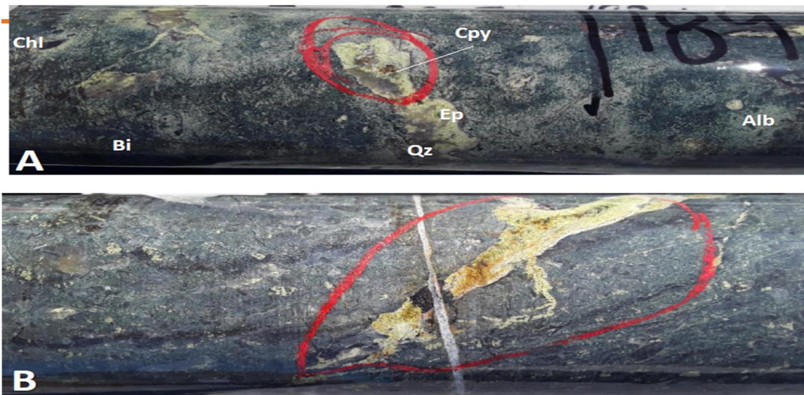
Figure 3: Hole MYLDH-005 -Examples of early biotite(Bi) +/- magnetite alteration overprinted by quartz(Qz)-epidote(Ep)-chlorite(Chl)-albite(Alb) +/- magnetite-chalcopyrite(Cpy) (A) and epidote-magnetite clot overprinted by hematite and native copper (B).
