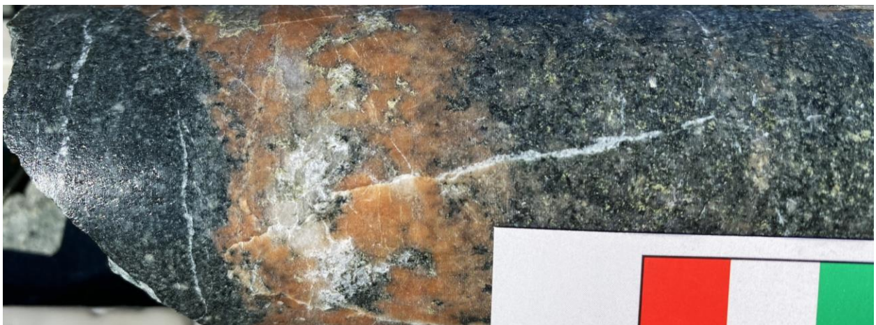
Figure 4: Photo of core from TRNDH002 (196.80m) showing pervasively chlorite-magnetite altered basalt with a crosscutting orange albite-quartz-carbonate-epidote-chlorite-pyrite-chalcopyrite vein.
