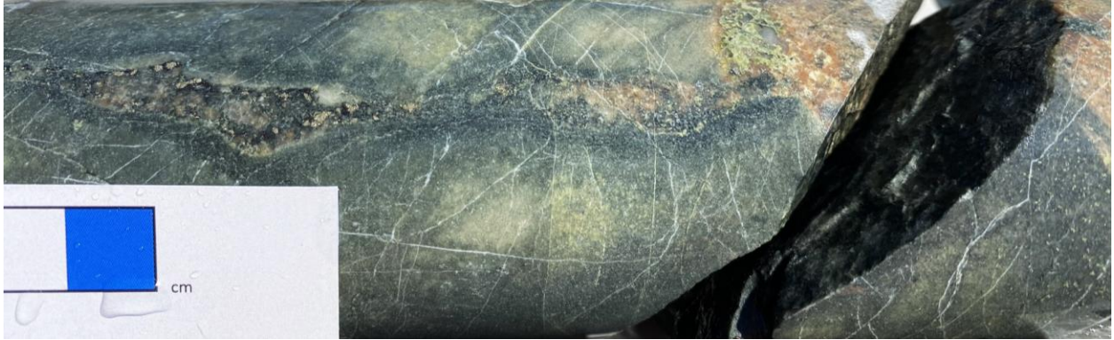
Figure 2: Photo of drill core from TRNDH002 (213.30m) showing complex multiphase alteration and veining associations. Early pervasive chlorite-albite-magnetite alteration overprinted by strong albite-epidote alteration further crosscut by complex quartz-epidote-albite-magnetite-chlorite-pyrite-chalcopyrite veins.
